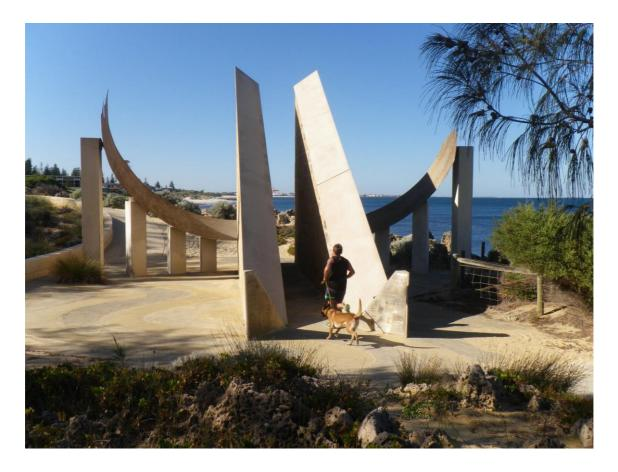
The Cottesloe sundial was built in 1993. It is based on 18<sup>th</sup> century sundials popular in Jaipur in India. The parallel triangular gnomons throw shadows onto engraved plates which curve on either side of them permitting accurate time to be read throughout the year. Curved lines engraved on the plates permit adjustment to WA standard time.
