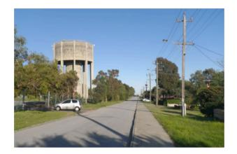
Gravity feed water tank that increases water pressure for the Perth suburb of Coolbellup.
