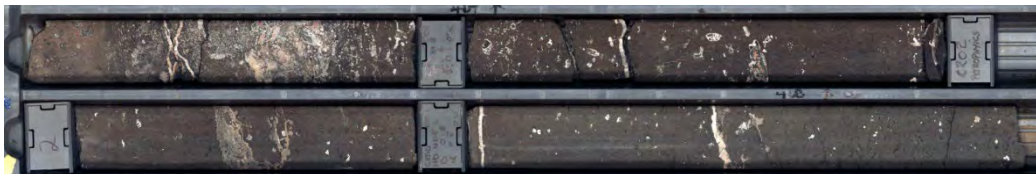
Rock core of a Kalkarindji lava flow (white dots were gas bubbles)
